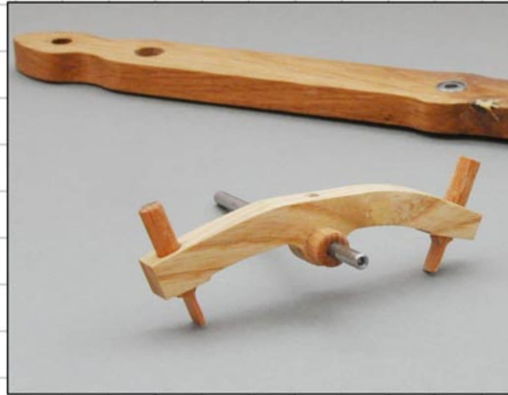
Assemble the Escapement and pallets to its shaft and initially set the protrusion of the pallets to the dimensions on the drawing, then fit to back panel.
