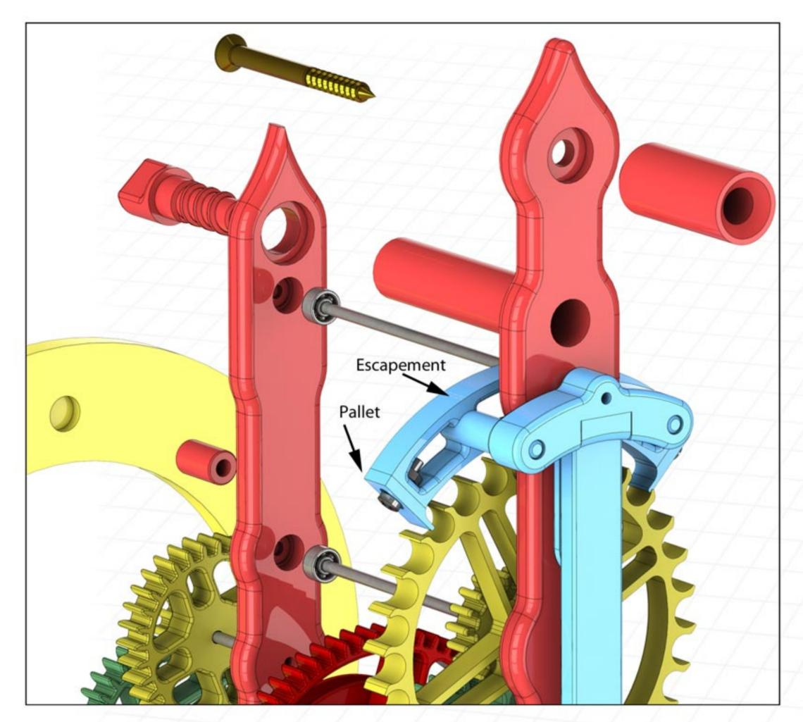
The Pallets are fitted to either side of the Escapement using a 2mm screw nut and washers. The The pallets are adjustable in and out to enable you to get the clock running evenly. If you start with the pallets fitted so that the top edges are level with the top edge of the escapement the clock should theoretically Tick Tock evenly . If it does, leave it at that setting, if it doesn't then start to adjust the pallets until it does.
