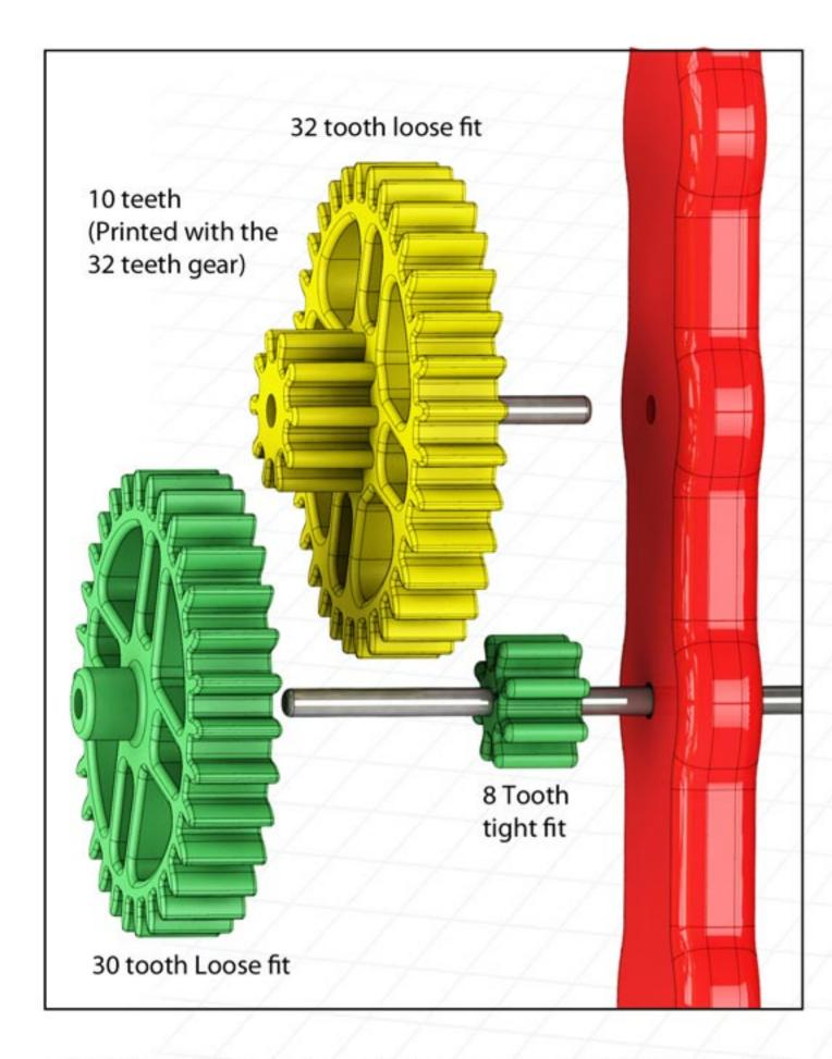
After fitting the front frame the hour gears can be fited to the two shafts protruding from the front face The 8 tooth gear needs to be tight to drive the others, but not so tight that you can't pull it off when you need to dismantle the clock.
