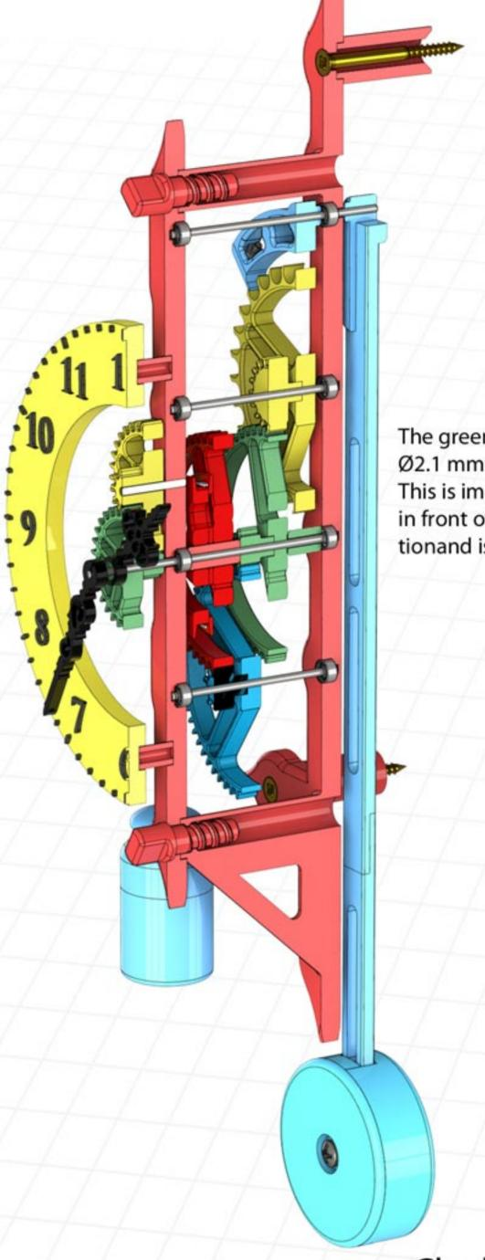
The green gear pair should be drilled out to Ø2.1 mm to be a free running fit on the shaft. This is importand as the red drive gear assembly in front of it is rotating in the opposite directionand is a tight fit on the shaft.
