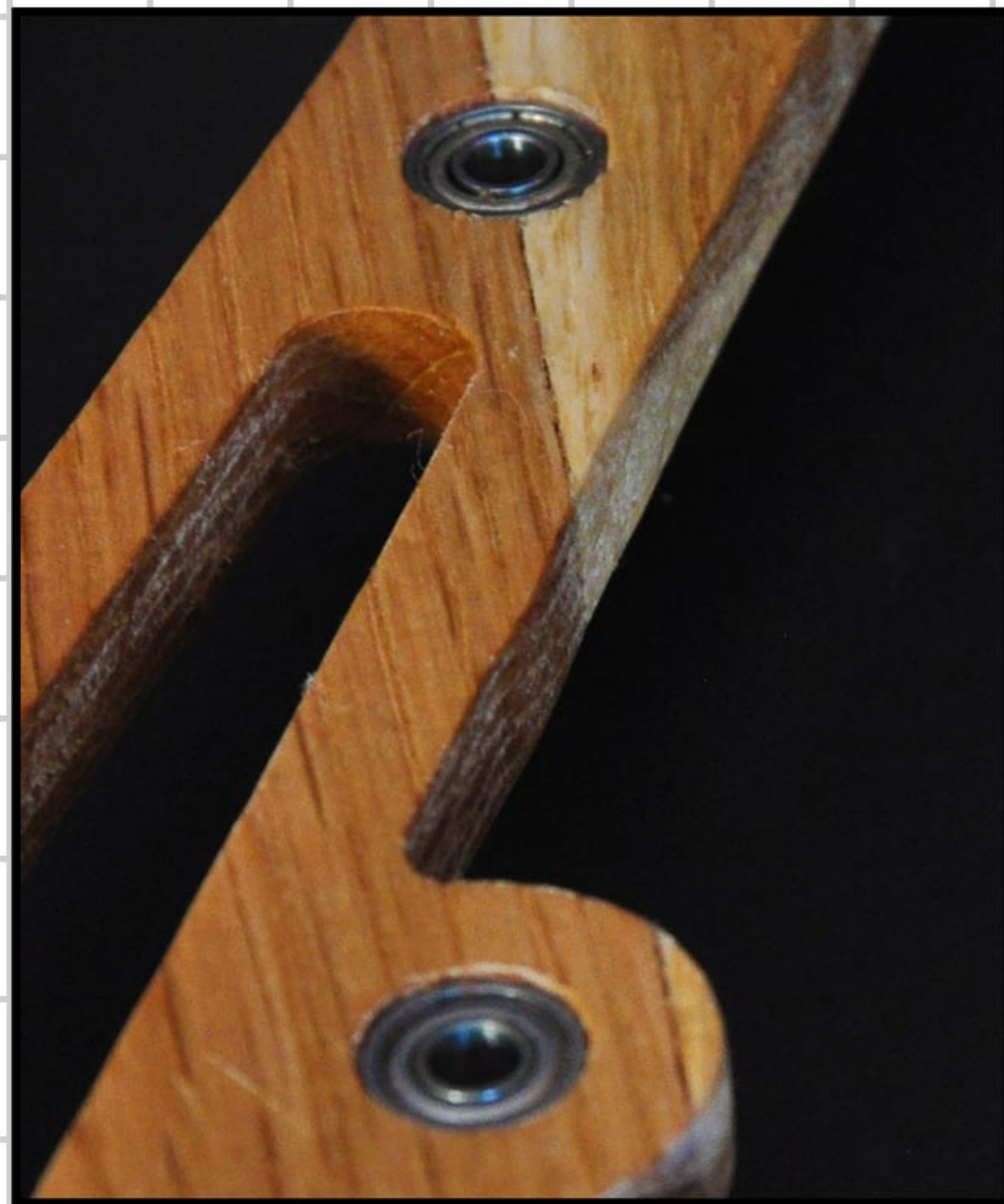
Fit bearings into front and back panels
