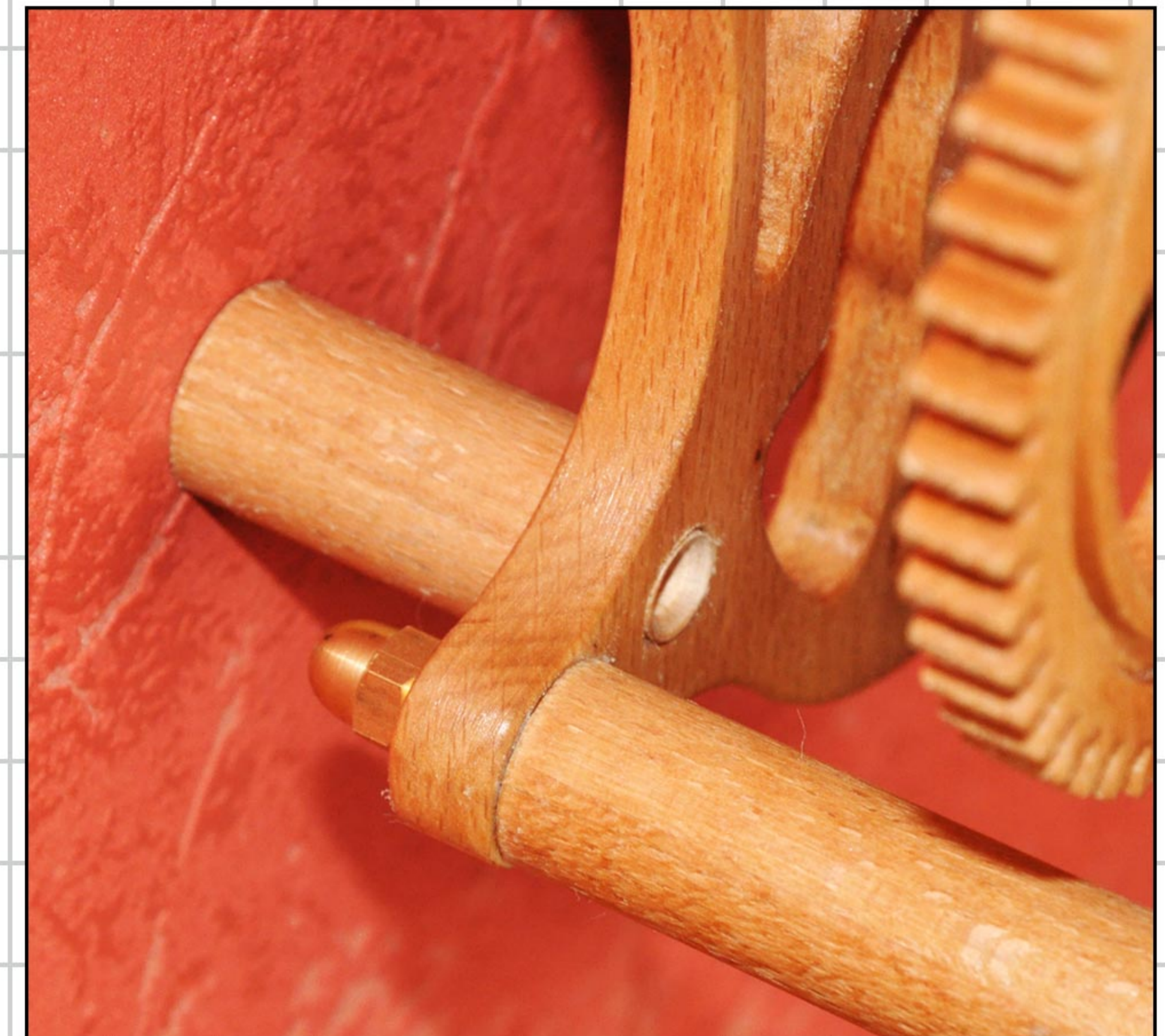
The bottom right support can either just rest against the wall as shown or be screwed to the wall.
