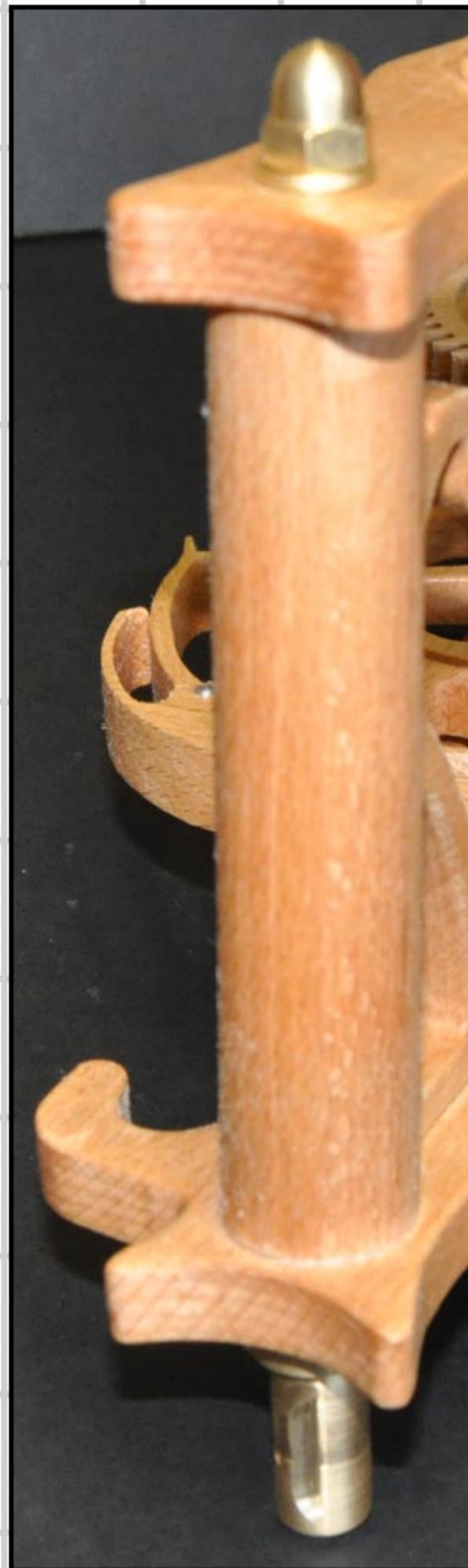
Fitting the Pendulum pivot and the domed nut
