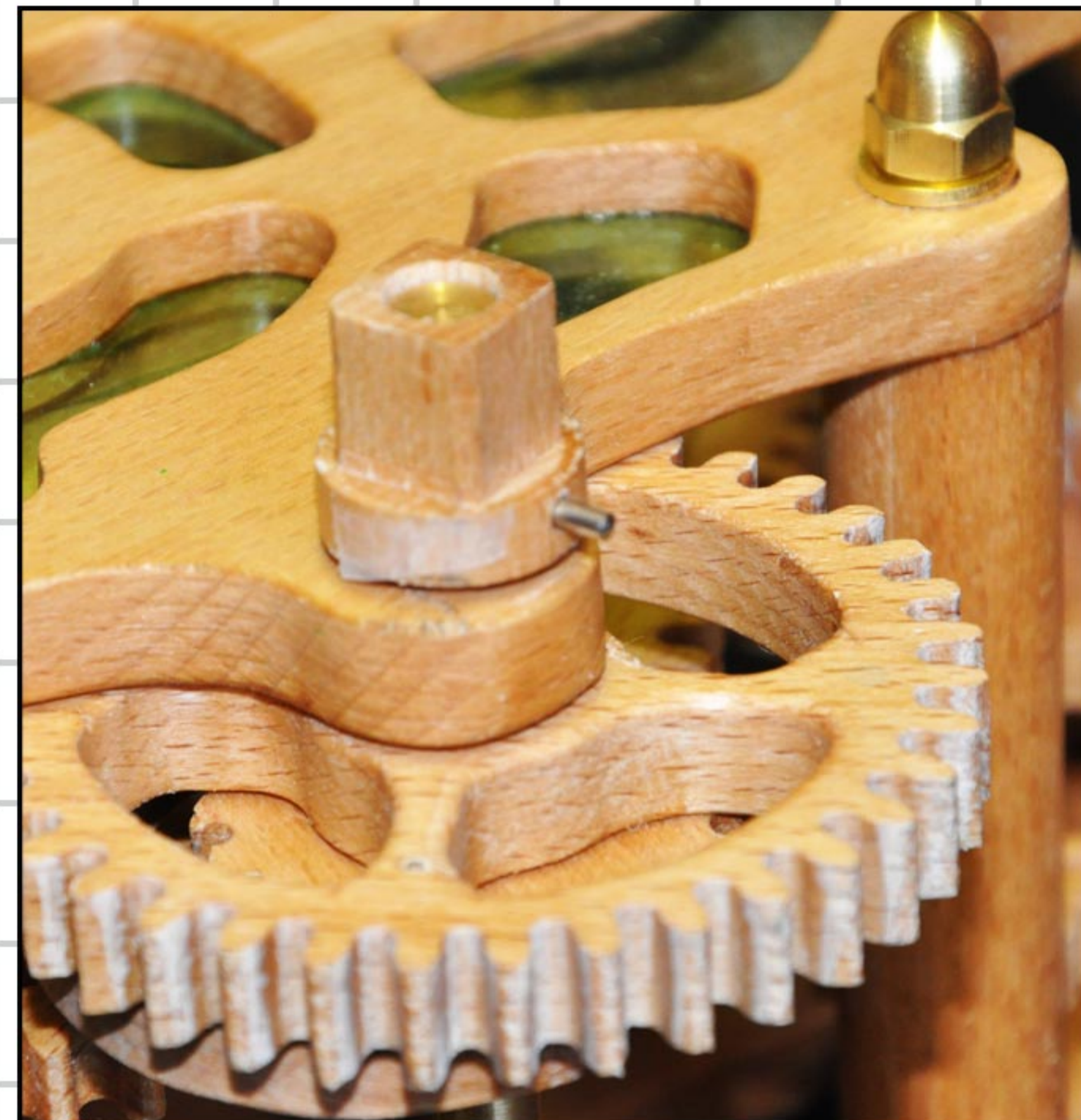
Fitting the Winder Stub using 2mm pin through the 8mm brass shaft
