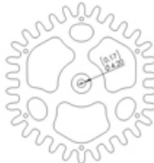
IX 47 Gear 30teeth 6 repeats Scale 1:1 8mm Thick
