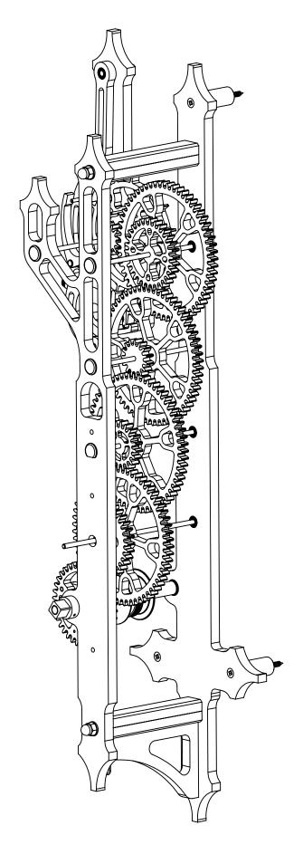
Brian Law's Wooden Clock 20 - Gravity Escapement Assembly Sequence Stage 6 Assemble Fit pendulum, mount on the wall . and fit weight to cord wrapped around the drum
