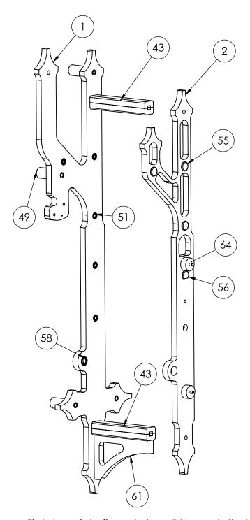
First stage is to fix and glue all the parts that are attached to the Front and Back frames.
