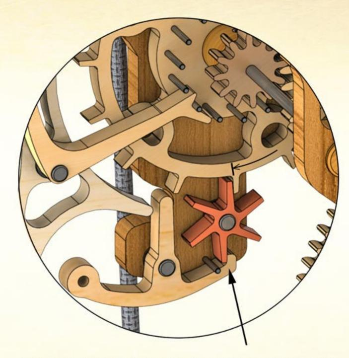
Escape wheel is driven by the gear train, but its rotation is stopped by the 6 legged Catch being held by the trigger.
