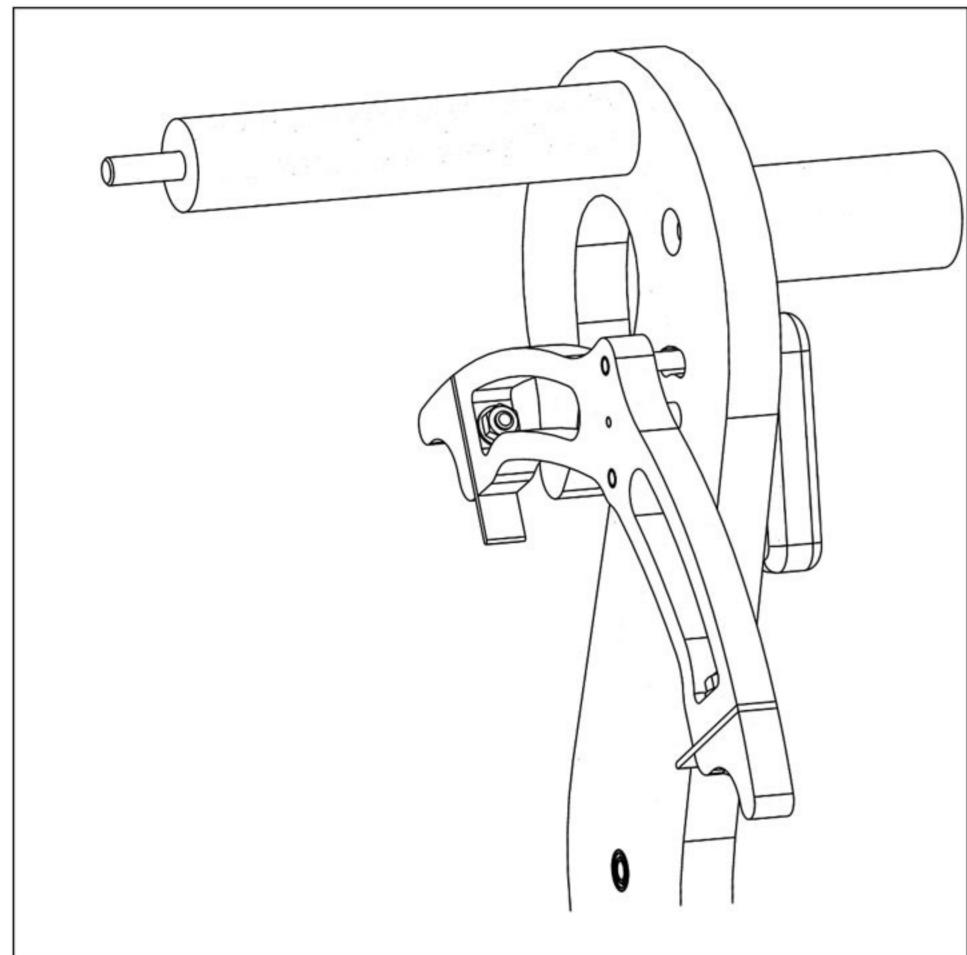
Pre Assemble the Pallets to the ends of the Escapement using the clamp pads and nuts and bolts.
