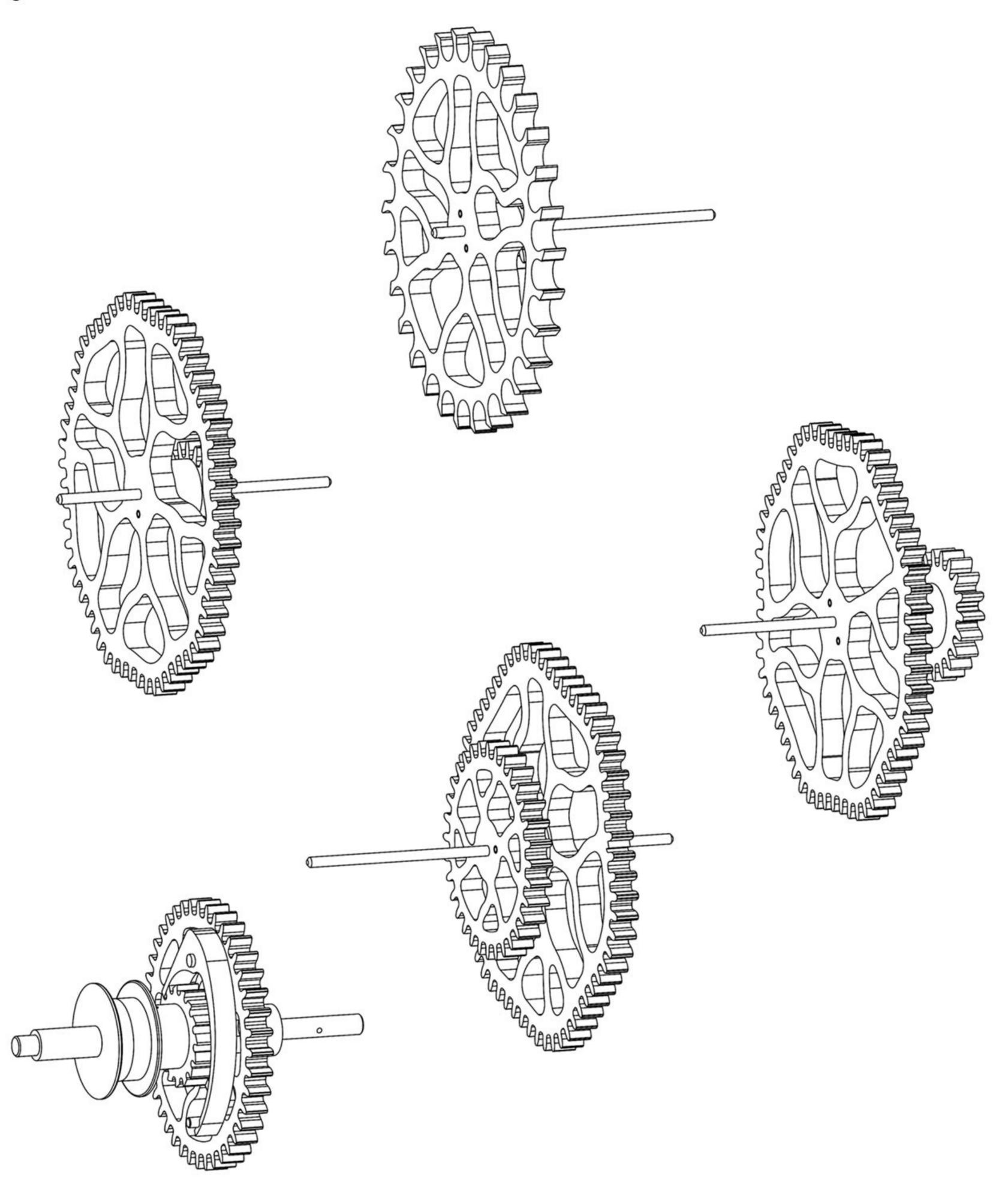
Assemble all Gear train Sub assemblies in accordance with the dimensions shown on the drawing Sheet . The Drive gear train shown at the bottom should have all the parts apart from the gear pinned to the shaft, the gear should turn freely and only be constrained by the ratchet from turning backwards. The other three assemblies should have the parts a tight fit on the shaft.
