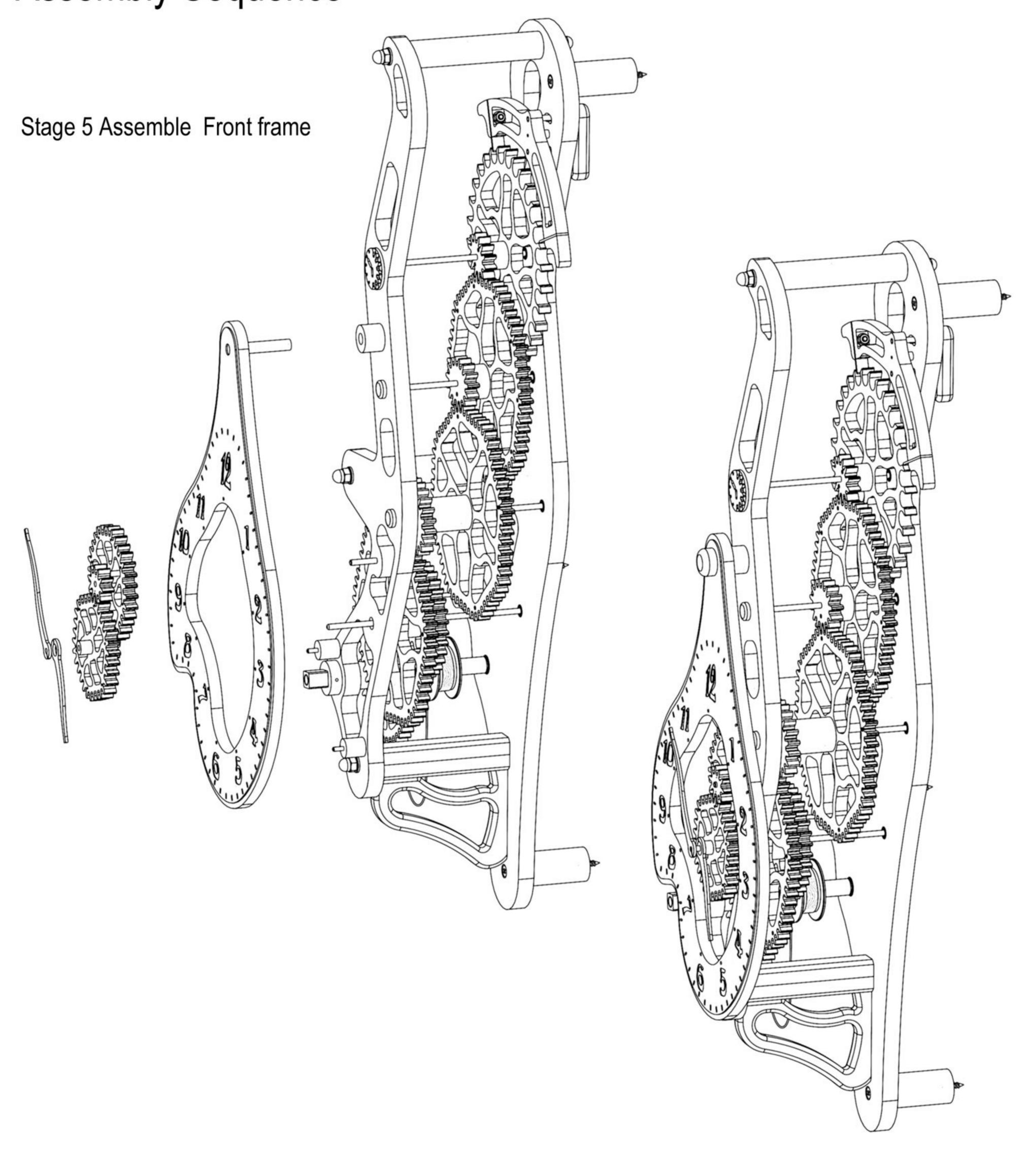
Fit the front frame taking care to align all of the shafts with the bearings and press down until the frame toushes on the frame spacers. Secure with dimed nuts and washers onto the threaded rods passed through the Frame spacers. The squre ended winder stub should be fitted to the end of the winder sub assembly after the front frame has been fitted, with a small 2mm pin. Fit pendulum, Hands and hour gears and mount on the wall.
