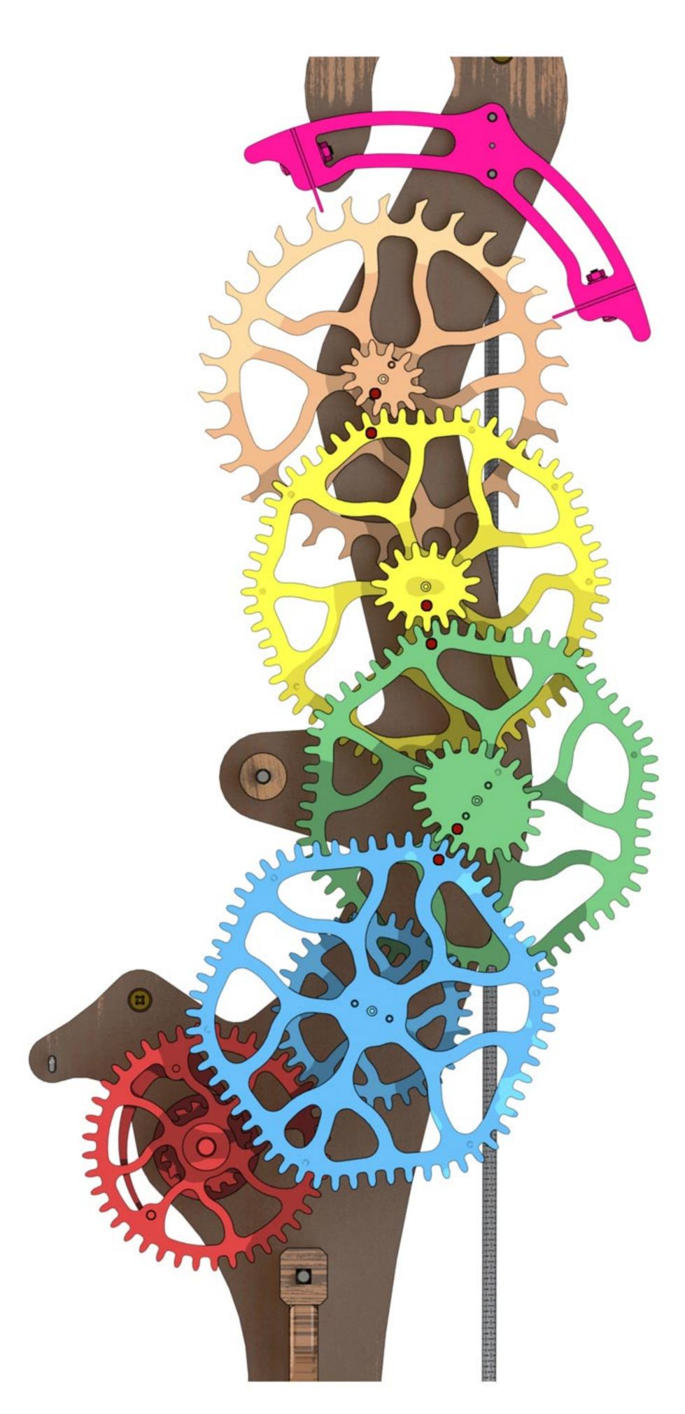
Fit the drive train gear sub assemblies to the back frame starting at the top with the Orange gears.
