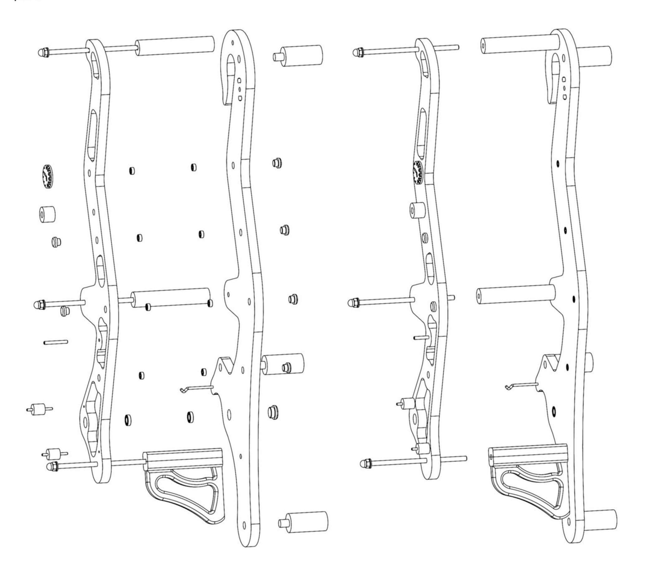
First stage is to fix and glue all the parts that are attached to the Front and Back frames. The bearing can be a tight press fit or be glued in place with Loctite. The Brace and the Spacers are glued to the Back Frame only.
