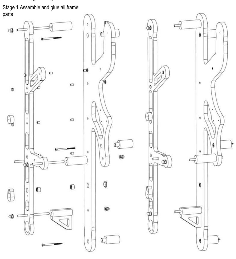
First stage is to fix and glue all the parts that are attached to the Front and Back frames. The bearing can be a tight press fit or be glued in place with Loctite. The Brace and the Spacers are glued to the Back Frame only.
