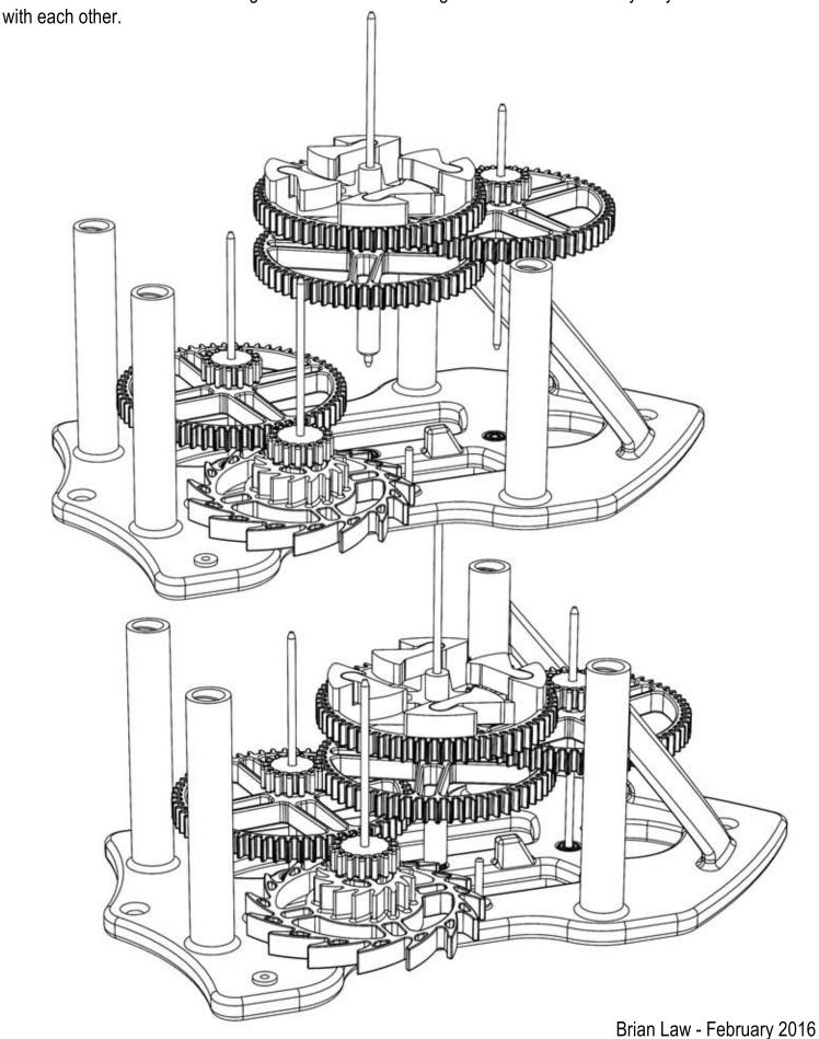
Stage Fit the ratchet with the cords wrapped around the pulleys in the manner shown
