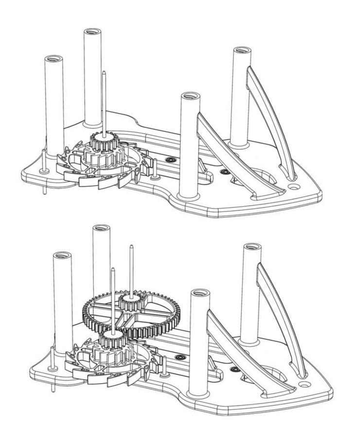
Stage Fit the bottom Intermediate gear and the two parts of the Drive Gear together as shown and then fit them into their bearings. You have to do this together because of the way they nest
