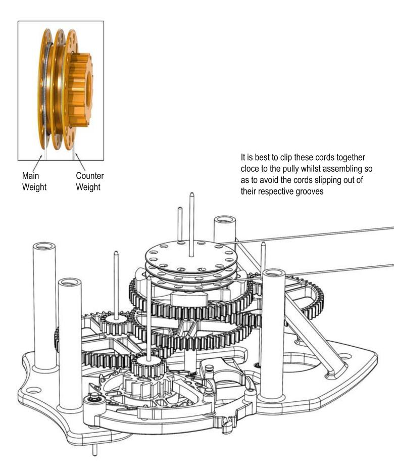
Stage Fit the Fit the assembled Gravity arm and the Trigger, and then the front Plated is lowered over the protruding shafts until it engages on the ends of the shafts, and then it can be screwed into position with the 4 plastic screws. Then fit the small 8 toothed gear onto the main shaft and push down until just clear of the Front plate.
