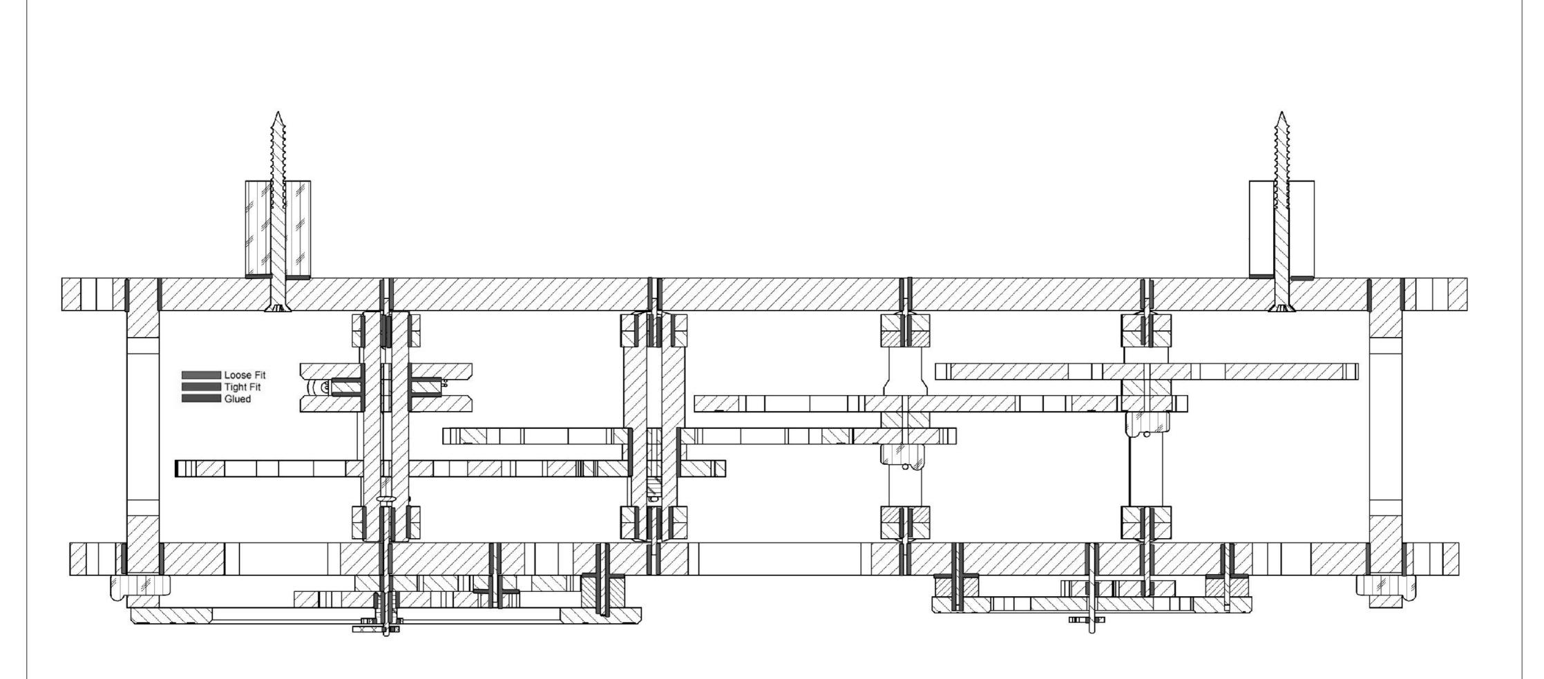
The section shown above is taken through the centre of the clock and shows all the shafts and the type of fits required.
