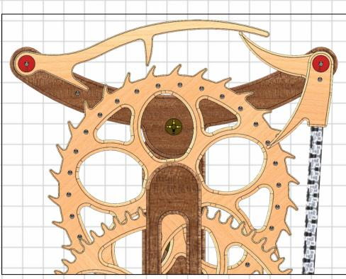
With the pendulum Hanging in the vertical position as shown on the previous page both the latch and the lower finger should be slightly engaged with the Pin and the Tooth. When the pendulum is swung it should produce an even Tic-Tock. If it doesn't then loosen the Fingers Support bar screw and move it slightly until the Tic-Tock is even, then tighten again.
