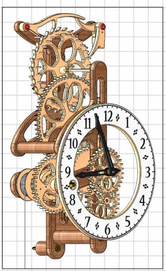
Mount the clock to the wall with the Back frame vertical and the Centre of the dial 1500 mm from the floor. Use the two woodscrews, one at the the bottom and one two thirds of the way up. Wrap the cord around the Drum making sure the end is secured to the drum with tape,
