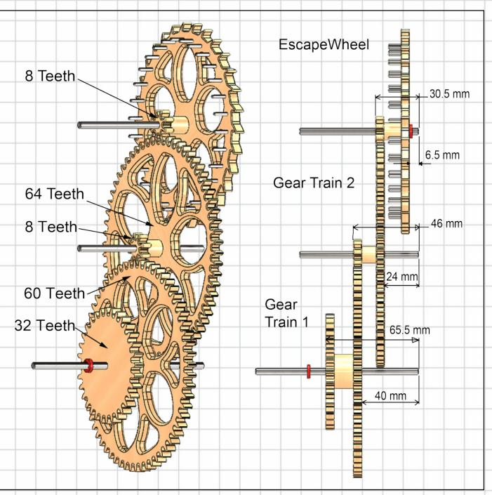
Assemble each gear train sub assembly in turn by driving the shaft through the centre holes in the spacers and gears. This should be done on a Drill press or similar setup to ensure the the shaft is fitted square to the gears. All gears should be a tight fit on the shaft and the gears and spacers should be glued together to ensure that there is no movement between the gears when a load is applied. The 30 pins fitted to the Escape wheel should be fitted first using the same Drill press setup.
