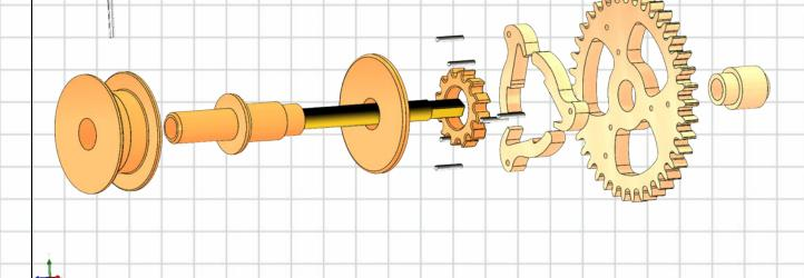
All the Orange parts should be glued together and then pinned to the Brass Drive shaft. The Pawl pins should be fitted to the holes in the 38 toothed gear. The drive gear spindle should be glued into the 38 toothed gear and be a loose fit on the Brass drive shaft. The Pawls are assembled onto the pins in the 38 toothed gear and gear and its parts slid onto the Brass Drive Shaft. Important Make sure that the ratchet and the Pawls are assembled exactly as shown above.
