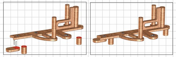
Now apply glue to the Backing plate and the tops of the two Wall spacers and stick to the underside of the Back frame. Use the Backing plate pins to locate the plate, use woodscrews to locate the Wall spacers.
