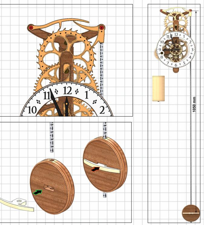
Make sure that the Finger support is horizontal and the securing screw tightened. Now Glue the Pendulum Rod into the hole in the Bottom of the Fingers part.
