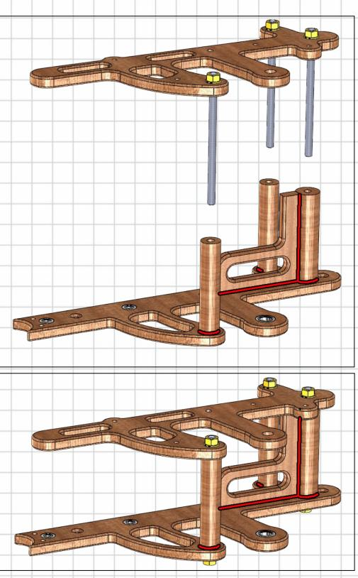
Glue the Frame spacers, and Brace to the front side of the Back frame as shown by the red lines and clamp both the Front and Back frames together using the Threaded rods and the M6 Nuts and Bolts to hold the frames accurately together as the glue dry's.
