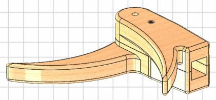
Fit the Finger pin into the Upper finger as shown and apply glue to the top face and then fit the two halves together. Fit a length of Ø2 rod temporally into the finger pivot hole to align the parts.
