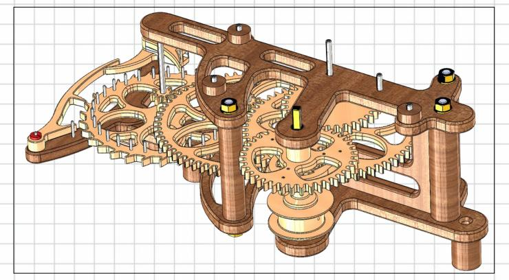
Fit the Front frame and secure with M6 Nuts and Bolts and Threaded rod
