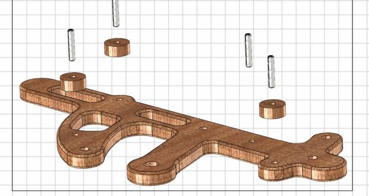
Fit the Dial Pins and spacers along with the Hour Gear Pivot pin to the front face of the Front frame. Spacers may be glued to the front frame if required.
