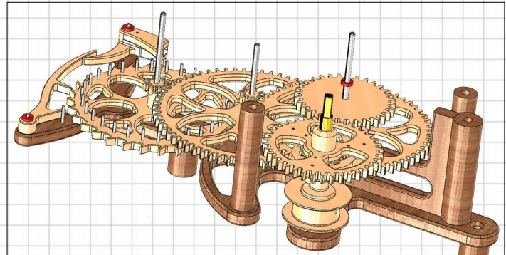
Finally fit the Drive Shaft assembly
