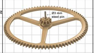
Drill through the spacer with Ø3.1 mm drill to produce a lose fit on the shaft. Drill and fit a 3mm pin into your bench and assemble and glue all the parts on to it. This should keep all parts square to pin
