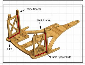
Fit and Glue the Frame spacers and the Frame spacer sides in place. Make sure they sit vertical by fitting the front frame temporarily
