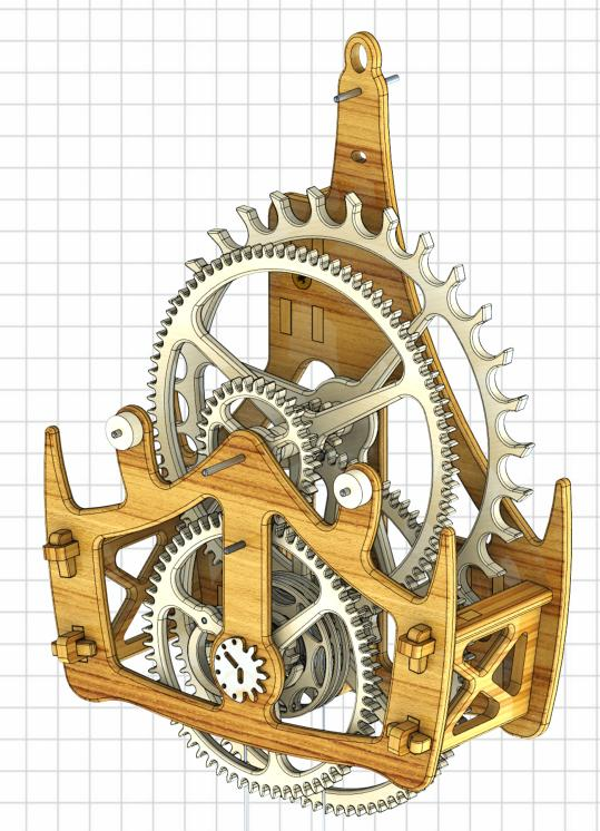
Fit the front frame by fitting over the 4 protruding Frame Spacers and engaging the the two protruding gear shafts. Secure in position with the four Wedges.
