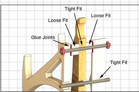
With the Escapement Arm and the Pendulum Assembled to the clock this cross section shows the fits required to allow them to swing together smoothly, the connector pin fitting loosely into the slot in the escapement arm ensures that his happens, it should not be too loose or too tight as this will prevent the impulse being transmitted to the Pendulum.
