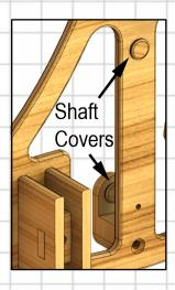
Shaft covers need to be fitted to the rear of the Back frame as well to prevent the shafts from protruding through the back face. This keeps all the meshing gears aligned.
