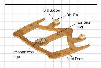
Start by fitting the 3 pins shown into the Front Front Frame and the placing the Dial spacers over the two top pins. The woodenclocks Logo acts as a shaft cover for the bottom shaft.
