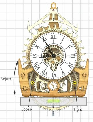
After assembling the clock and fixing the Cord the clock can be mounted horizontally onto the chosen wall with the centre of the Dial at a height of around 160cm this should give a running time around 24 hours.
