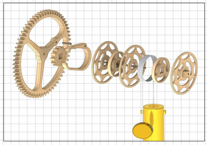
You will need to study the detail drawings to see a description of all of the parts in this sub assembly, it is the most complicated of the sub assemblies used on the clock, Take a special note about the fitting of the Pawl and the orientation of the ratchet.
