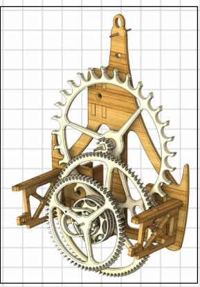
Load each of the Gear and Escape Wheel sub assemblies into the Back frame in the sequence, it is best to do this with the clock laying down on its back. Fit the Escape wheel first using the shaft to hold it in place. Next place Gear train2, followed straight the way with the drive assembly which has the shaft already fitted to it. Now place the Gear train 1 Assembly onto the top shaft shown in the illustration below.
