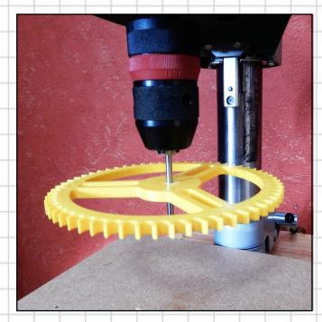
The Drive train sub assemblies shown above are all very similar and require to be assembled in the same manner. I recommend you use a drill press to do this as I have done, as it ensures that the gears are all mounted square to the shaft,. They should all be a Free wheeling on the shaft except for the **Gear train 1**. Make sure to glue all gears and spacers together so there is no relative movement between the parts.
