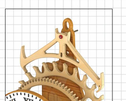
Glue the Escape arm Sleeve to the Escape arm making sure to keep the two parts properly aligned whilst the glue dries, by sliding a shaft in place between the two of them.
