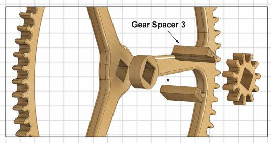
Glue together the 2 parts of Gear Spacer 3
