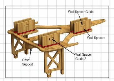
Fit the pairs of Wall spacers and their guides together and then glue in place to the back of the Back frame. Note the Wall spacer Guide 2 is free to move up and down a bit to aid aligning the clock on the wall.
