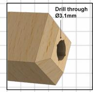
Geartrain1 needs to be a tight fit on its shaft
