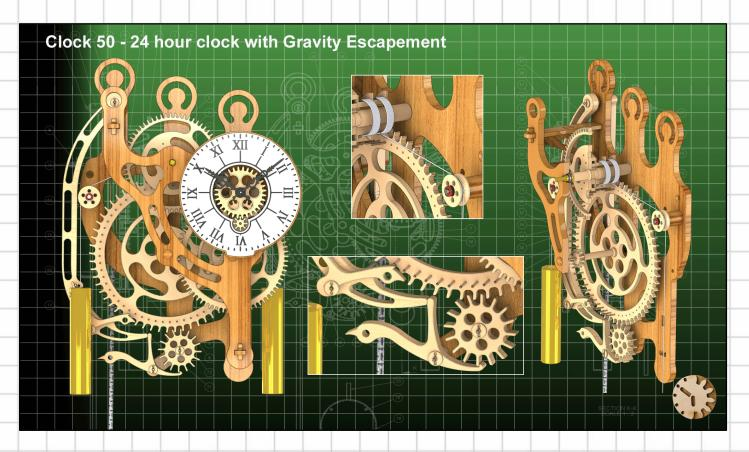
The prototype for Clock 50 is now completed and running really well, it uses the woodenclocks Gravity escapement and runs for 27 hours on a wind. It has 2 driving weights 750 gram each and the reason for splitting the weight like this is to remove the load from the Front frame and stop Parallelogram distortion. It does add to the complexity of the clock but the benefits in terms of reducing structural load are worth it.
