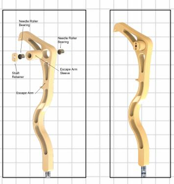
First fit the 2 Needle roller bearings into the Sleeve, one in each side. Then fit the sleeve into the top of the Escapement Arm, gluing in place. Now Slide the Pendulum Rod into the hole in the underside and glue into position if it is not a tight fit.
