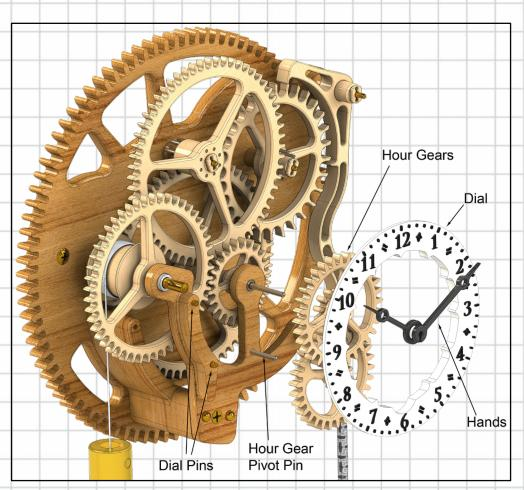
Fit the front frame by fitting over the 2 protruding 6 mm diameter pins and engaging the the 2 protruding gear shafts.
