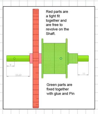
The drum is the first to be fitted and glued to the Drive Spacer and then fitted to the drive shaft by drilling and pinning with the Drive Pin in the position shown on the left here.
