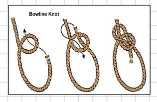
With the Cord hanging down to the left of the drum tie a loop in the end of the cord using a Bowline Knot or similar. Now attach the weight by pushing the Loops into the hole in the top and securing by sliding the weight hanging pin through the holes in the side at the top. The clock should now start running.
