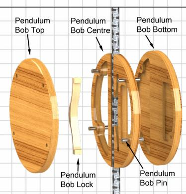
To assemble the Pendulum Bob First fix the Top and the Centre parts together using the 4 pins, then lay the Ball bearings into the pockets to get total weight around 150 grams. Fit the lock in position and fit the top part, then slide onto the pendulum Rod. (Note! The Ball bearings are not shown, any size can be used that fits)
