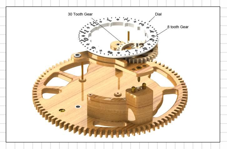
Finally for this stage glue the 8 toothed gear to the top of the 30 Toothed gear and ensure the centre holes are lined up before it dries, Drill out afterwards to ensure the pair of gears run freely on the Pivot.
