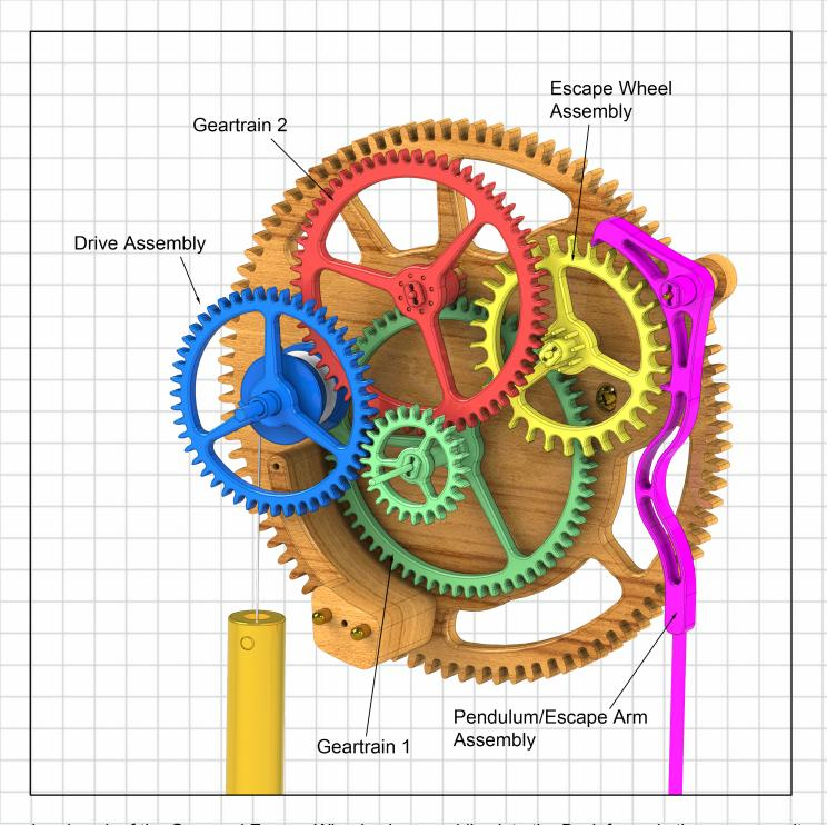
Load each of the Gear and Escape Wheel sub assemblies into the Back frame in the sequence, it is best to do this with the clock laying down on its back. Fit the Geartrain 1 first, next place Escape Wheel, followed straight the way with the Gear train 2 and finally Drive Assembly. Now load the Pendulum assembly finally wind the cord onto the Drum, Winding clockwise when viewed from the front of the clock.
