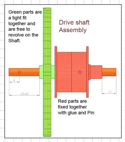
The Drum and the Spacer need to be drilled on assembly and the fitted with the Pin to lock the Drum securely to the shaft. Care should be taken to maintain the 11 mm dimension of the drum to the end of the shaft.
