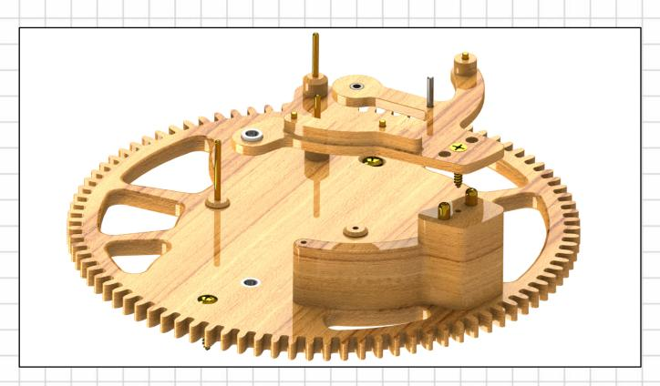
Start by fitting the 2 Needle Roller bearings into their respective holes ,note that the Larger bearing sticks out 3 mm either side of the front frame Now fit the 3 Dial pins shown into the Front Frame, along with the Hour Gears Pivot pin.
