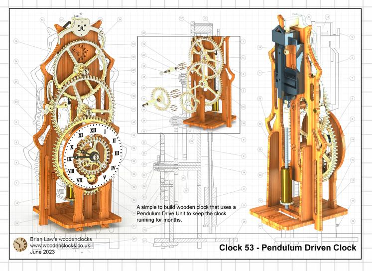
Over the last 30 years I have been designing and building wooden clocks and the one thing that they all have in common is they are entirely mechanical with no electrical or electronic drive systems, they either use a weight or a powerful spring to drive them. That is going to change on this next clock with the introduction of a Pendulum Drive Unit usually used along with a quartz powered motor to drive the hands of a clock.
