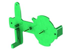
We will start assembling the Back Frame by press fitting the two shafts into the front face of the Back frame. The missing shaft will be fitted later as this is to be a lose fit into the support pillar. Next glue the Wall Spacers and the Drive Support in position on the back face, using the screws to align the holes. Note the Drive support fits into the shallow recessed slot on the rear. The blue lines indicate where to glue.
