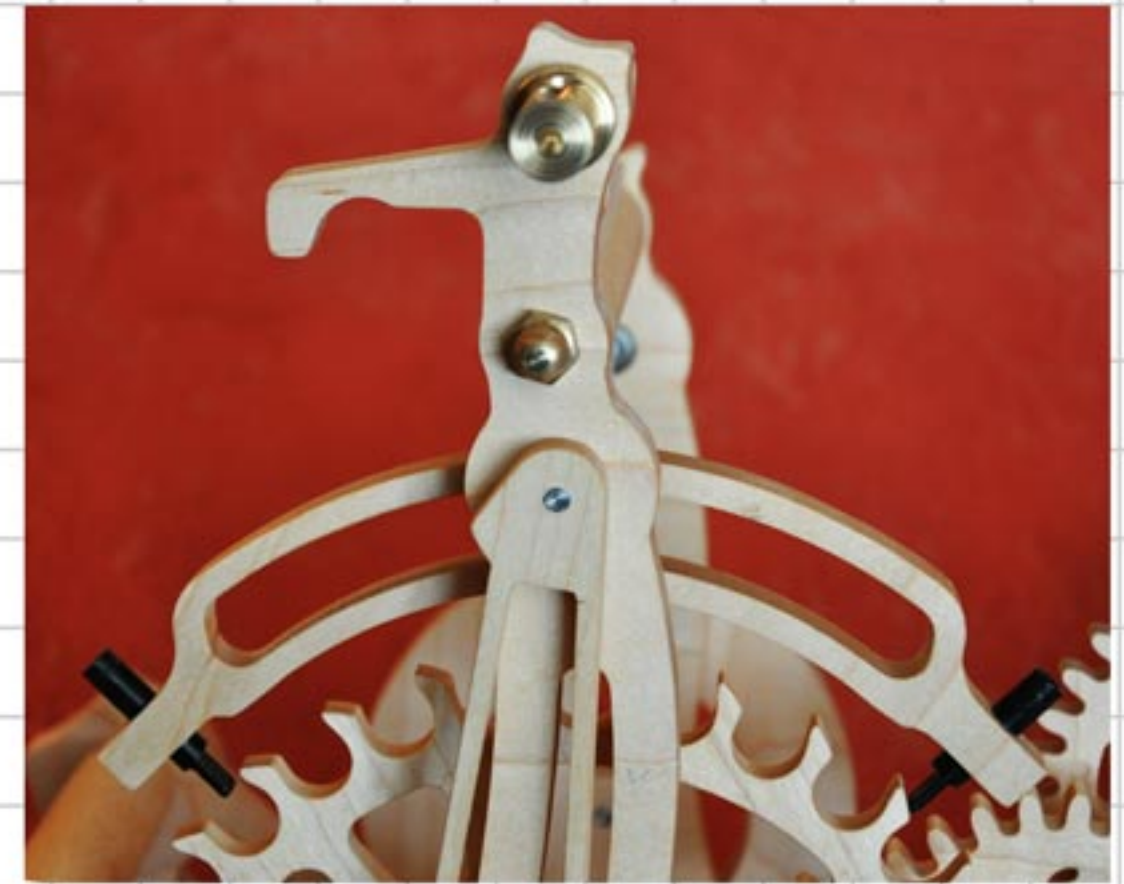
Fit the Pallets and adjust so that they protrude 11 mm below the underside of the escapement
